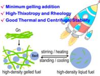
Four kinds of gelled high-density fuels formed by  $SiO_2$  and Gn were synthesized. Compared with  $SiO_2$  gelled hydrocarbonfuels, Gn gelledhydrocarbon fuels show higher thixotropy and rheology, along with better thermal and centrifugal stability. Additionally, the addition amount of Gn for gelling the fuels is not greater than 1% with little influence on the density and heat value of the fuels.
