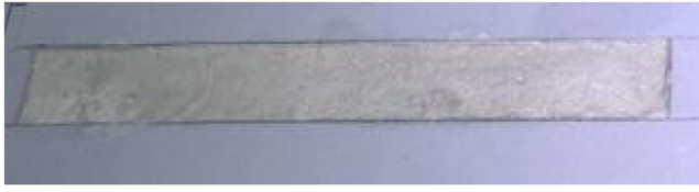
Fig.5 A sample of the film charge of the VS-2 pyrotechnic composition
