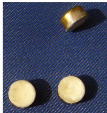
Fig. 4 External view of assemblies of VS-2 pyrotechnic composition charges
