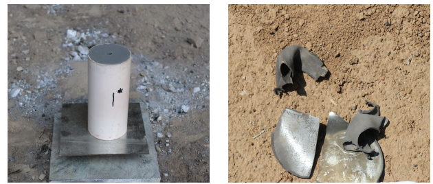
a. test device before test b. witness plate wreckage after test
