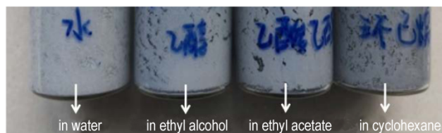
图2 FB-03经不同溶剂超声分散浸泡清洗30 min后实物图 Fig.2 Photos of FB-03 after ultrasonic dispersion immersion cleaning for 30 min in different solvents
