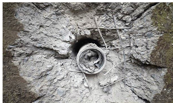
a. penetration of test projectile into concrete target
