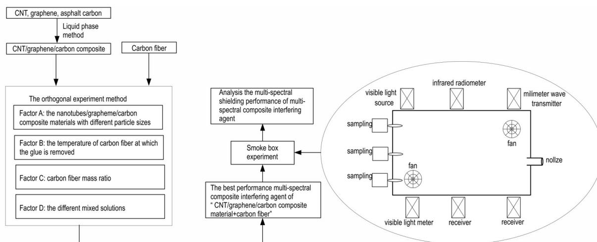
The carbon nanotube/graphene/carbon composites prepared by liquid phase method and the carbon fiber were used to prepare the better shielding performance interfering composite in proportion by the orthogonal experiment method. Based on the smoke box experiment, the shielding performance of the interfering composite, and the influence of various factors were further analyzed.
