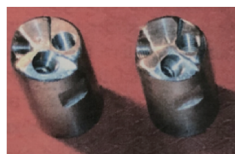
Fig.2 Cavitation nozzle
