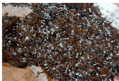
b. carbon fiber roasted at 400\ ^\circ\text{C}
