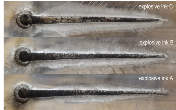
图6 三种炸药油墨样品临界传爆厚度测试结果 Fig.6 Critical detonation thickness test results for three explosive ink samples
