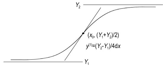
Fig. 2 Typical S-shaped curve and physical significance of parameters
