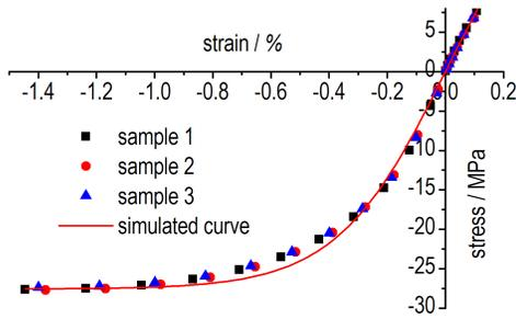
**Fig. 5** Comparison of the the tests and simulated curve by the two-parameter Boltzmann constitutive model with parameter values based on analytic results at 20 °C
