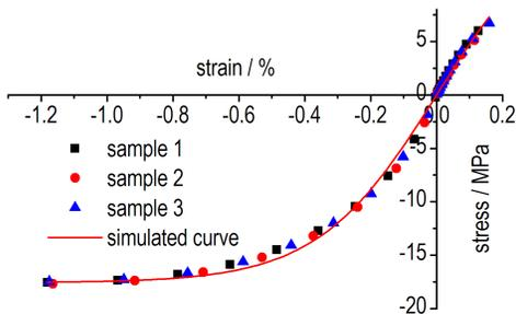
**Fig. 7** Comparison of the tests and simulated curve by the two-parameter Boltzmann constitutive model with parameter values based on analytic results at 50 °C
