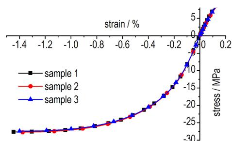
Fig. 1 Tension-compression stress-strain curves of PBX-901 at 20 °C
