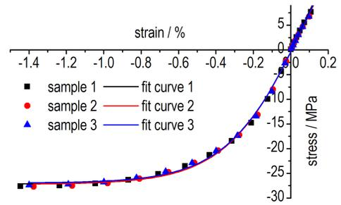
Fig. 3 Comparison of the tests and fitting results of the four-parameter Boltzmann constitutive model of PBX-901 at 20 °C
