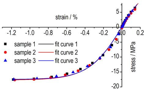
**Fig. 6** Comparison of the tests and fitting results of the two-parameter Boltzmann constitutive model of PBX-901 at 50 °C
