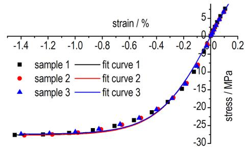
Fig. 4 Comparison of the tests and fitting results of the two-parameter Boltzmann constitutive model of PBX-901 at 20 °C
