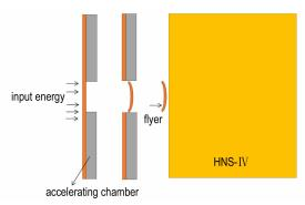
The process that bridge foil driven flyer to detonate HNS-IV was simulated by ANSYS/AUTODYN software. The influence of bridge foil thickness on flyer speed was studied, and the influences of bridge area width, flyer material, flyer thickness and accelerating chamber length on EFI ignition threshold were investigated.
