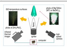
The influence of different ignition agents and orifice diameters on the combustion and expansion characteristics of the base bleed igniter burning in the atmosphere was experimentally evaluated by HSC and ITI analysis. A three-dimensional simulation of the burning jet of MT igniter was conducted.
