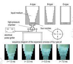
To explore the method of controlling the combustion stability of bulkloaded propellant guns, we design the experiment to study the expansion characteristic of four combustion-gas jets in five-stage cylindrical stepped-wall type observation chamber with different parameters.
