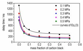
The effect of mass fraction of carbon black on the ignition and combustion characteristics of polyethylene under environmental pressure was studied. The ignition process, ignition delay time and burning rate of solid fuels under different environment pressure were discussed. Based on experimental data, mathematical relationship between ignition delay time and mass fraction of carbon black was given by using the least squares method.
