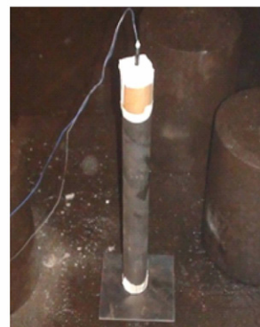
Fig. 1 Schematic showing of the UN gap test
