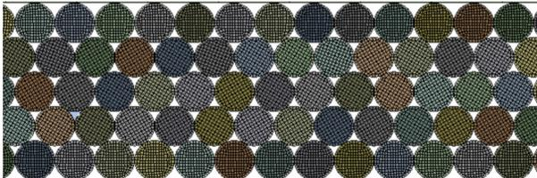
Fig. 6 Magnification of mesh of HMX particles
