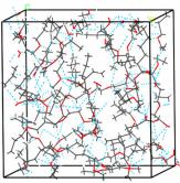
The compatibilities of HTPE with DBP, DOS and DEP were studied by molecular dynamics simulation method. By analysing the binding energy, radial distribution function and glass transition temperature, the compatibility of the polymer binder with the plasticizer could be predicted.
