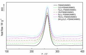
Effects of CuO,  ${\rm Fe_2O_3}$ , CB,  ${\rm PbCO_3}$ ,  ${\rm Bi_2O_3}$  and  ${\rm (NH_4)_2Cr_2O_7}$  on the thermal decomposition properties of P (BAMO/AMMO) energetic binder were studied by TG and DSC.
