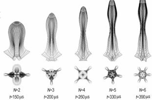
Multi-point initiation explosively formed projectile (EFP) charges with different N (the number of initiation points),  $D_1$  (the diameter of annular initiation),  $L_c/D_c$  (the length/diameter of charge) were studied by LS-DYNA program. Shapes of EFP with fins formed by different numbers of initiation points (N=2-6) were approached by numerical simulation. The number of fins was equal to the number of initiation points.
