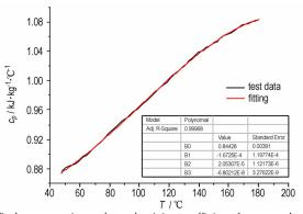
The specific heat capacity and conductivity coefficient for unaged and naturally aged (stored in a sealed plastic bag under room temperature) AP/HT-PB base bleed propellant used in a 155 mm base bleed projectile were determined by differential scanning calorimeter (DSC) and conductometer.
