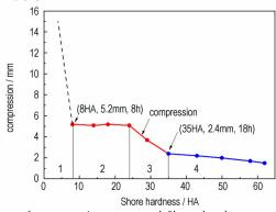
The influence of compressive stress and Shore hardness on the annular gap defect of a casting polymer bonded explosive (P-1 explosive) charge after curing was studied using a compression technology. The relationship between stress and strain was analyzed. The fitting equation of stress-strain for P-1 explosive in compression curing process was obtained. The CT detection of the explosive was carried out.
