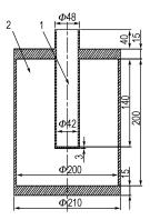
The double-layer test device filled with different gases was used to study the effects of the explosion energy outputs of thermobaric explosives under closed condition. The experiment was studied by an underwater explosion test method, the inner container was used to place the explosives, and the outer container was used to fill different gases under different pressures.
