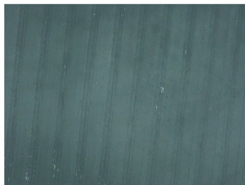
b. the surface morphology of RDX single crystal (50 ×)
