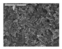
The ultra-fine 2, 2', 4, 4', 6, 6'-hexanitorstilbene (HNS-IV) was prepared by using solvent/anti-solvent recrystallization method. The effects of solvent factors, drying methods and process parameters, including the different solvents, anti-solvents, washing solvents, temperature, drying methods on the average particle size, particle size distribution and morphology of HNS, were studied.
