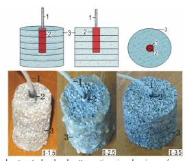
In order to study shock attenuation in aluminum foams, the different thickness of aluminum foam shells were made, shock attenuation in its was preliminarily investigated. Two types of PETN charges were used, one is the PETN itself, the others are confined by aluminum foam shell with thickness of 1.5 cm, 2.5 cm and 3.5 cm. The shock wave pressure-time curves were obtained at 0.5 m away from the charge.
