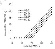
Effects of dibutyl phthalate on combustion carbon residue of doublebased propellant was studied by using computational method of minimum free energy. The function of the critical value of dibutyl phthalate content and the nitroglycerine content, combustion pressure was established based on the computational results.
