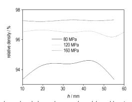
The polymer-bonded powder was shaped by rubber isostatic pressing (RIP). The higher the pressure, the better are the properties of compact. At the pressure of 160 MPa and initial relative density of 62%, the axial density difference of compact is less than 0.4%, and the RIP tends to isostatic pressing and becomes a net shaping process.
