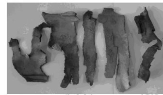
a. fragments produced by the 3 mm-thickness shell
