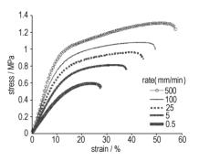
The influence of strain rate and loading on tensile properties of HTPB propellant was studied by means of uniaxial tension and cycling loading. The dissipated characteristics under mechanical loading was analyzed based on dissipated energy model. The relationships between tensile strength, elongation, dissipated energy and the logarithm of strain rate were created by linear regression.
