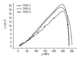
Effect of particle size and types of nitramine on combustion performance of energetic thermoplastic elastomer (ETPE) gun propellants based on BAMO-AMMO were studied by closed bomb test.
