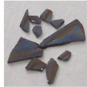
a. exploded pieces of porous silicon energetic chips
