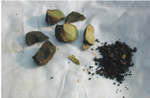
b. recovered fragments and black gelatinous granules of explosive in Test 1
