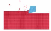
Numerical simulation of HMX based PBX explosive machining was performed by using LS-DYNA. The computing model, materials model and chip separation criteria were studied and presented.
