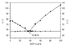
High energy density material DNTF can form eutectic mixture with TNT.
