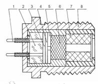
YANG Zhen-ying, CHU En-yi, Lü Qiao-li, REN Xi, GAO Fu-ping, REN Ling *Hanneng Cailiao*, 2004,12(1): 56 The exploding foil igniter consists of slapper igniter and ignition composition cup. The in-line ignition train permit composition was used in the charge. The performance was studied. The ignition joint test to rocket motor ignition composition was successful.
