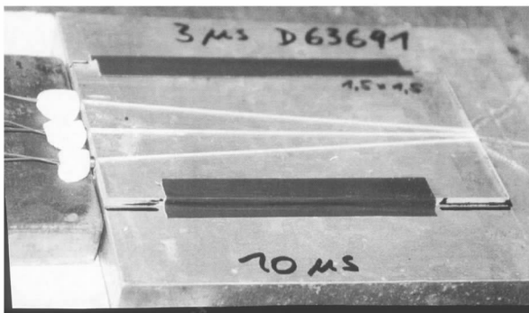
Fig. 7 Arrangement of the V-shaped traces with the detonators on the left side on a 10 mm thick aluminum plate
