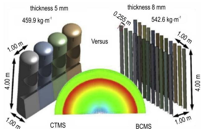
图 13 CTMS 和 BCMS 抗爆墙<sup>[109]</sup>Fig.13 CTMS and BCMS blast wall<sup>[109]</sup>
