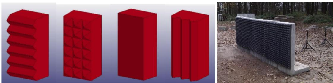
图6 波纹型和角锥型抗爆墙<sup>[71,84]</sup>Fig.6 Corrugated and conical blast walls<sup>[71,84]</sup>
