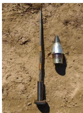
c. strain gauge pressure bar sensor and Fuse
