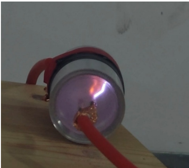
图 10 电击穿过程电弧现象 Fig.10 Photo of the electric arc phenomenon during electrical breakdown process
