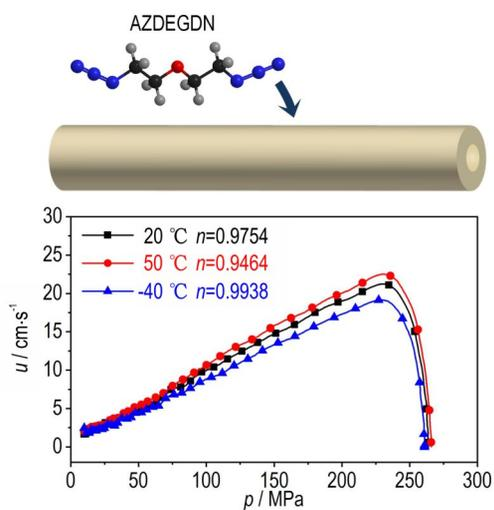
Double- and triple-base gun propellants containing a novel azido plasticizer 1, 5-diazide-3-oxapentane (AZDEGDN) were prepared by a semi-solvent method for the first time, and the static combustion performance of AZDEGDN-containing propellants at different temperatures was thoroughly studied by closed vessel tests, which will promote the application of new azido plasticizers such as AZDEGDN in low-ablation gun propellants.
