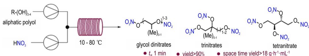
图 14 硝酸酯的连续合成工艺流程图<sup>[64]</sup>Fig.14 Flow chart for the continuous synthesis of nitrates<sup>[64]</sup>
