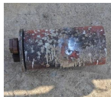
b. test shell with venting hole
