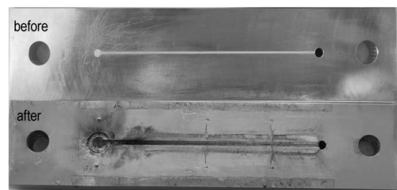
b. comparison before and after the explosion velocity test
