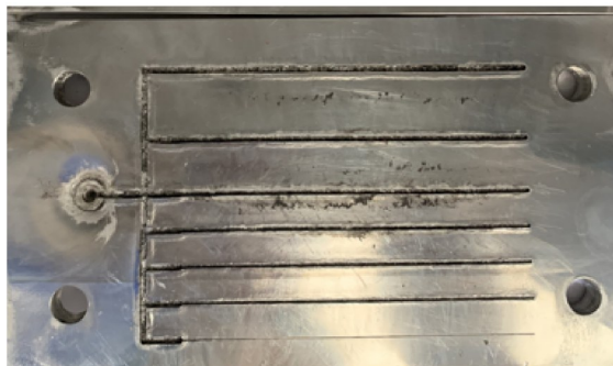
b. optical images of workpiece after critical detonation size test of printed sample
