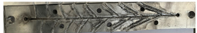
b. optical images of workpiece after detonation corner turning test of printed sample
