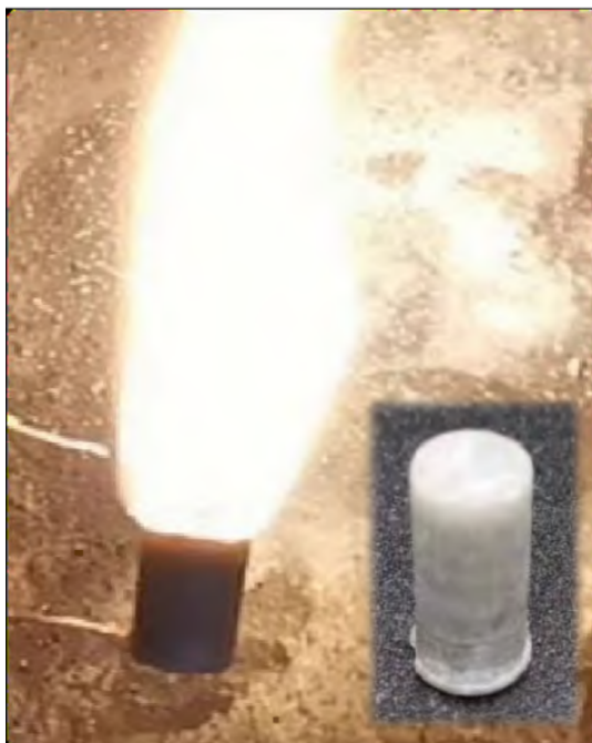
Burning process of delayed energetic grain
