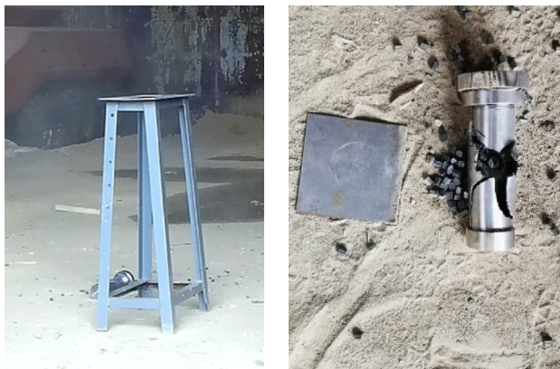
a. the state after the cook-off bomb and witness plate fell to the ground b. cook-off bomb and witness plate
