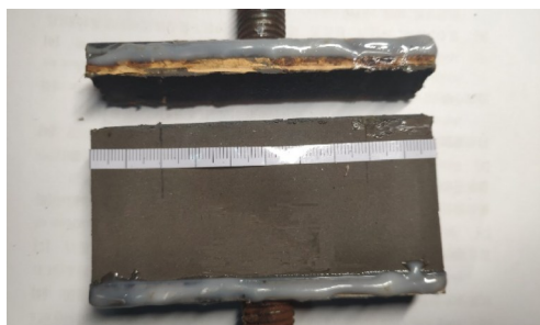
b. the interface layer is obviously stratified
