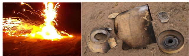
图4 大尺寸固体火箭发动机试验过程及残骸 Fig.4 Experimental process and wreckage of full-size SRM
