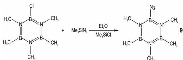
Scheme 24 Synthesis of 6-azido-1, 2, 3, 4, 5-pentamethylborazine (9) [37]
