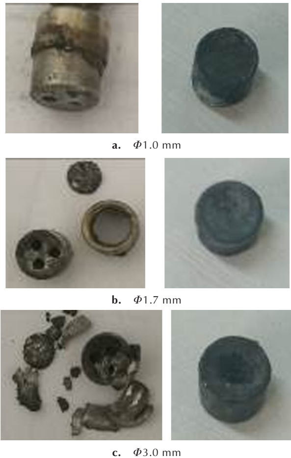
图 8 不同直径击针撞击后火帽破坏和铅柱受冲击情况 Fig. 8 The damage of primers and impact situation of lead pillars after the impact by firing pins with different diameters
