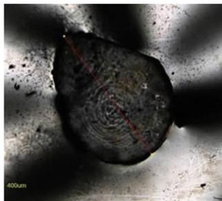
d. Cr/Al flyer prepared by electron beam evaporation
