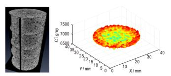
Three dimensional visualization of 2, 4, 6-triamino-1, 3, 5-trinitrobenzene (TATB) molding powder under isostatic warm compaction was performed using X-ray microtomography (X- $\mu$ CT). It allows a quantitative analysis of the compacted granules, including the size distribution and CT value variance in different slices.
