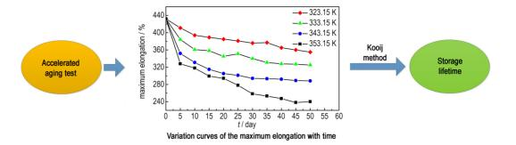
Accelerated aging tests at 50, 60, 70 °C and 80 °C were conducted, and the maximum elongation of the aging HTPB coating was tested. The experimental data were used to solve the Kooij model, which predicted the storage life time of HTPB coating at 25 °C.
