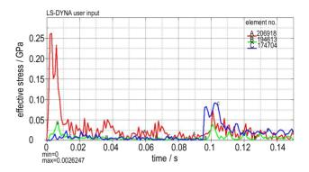
The drop process of solid motor at different angle was analyzed. The stress in propellant can reach a few hundreds megapascal. Data information from the drop test of solid rocket motor is similar to the results of finite element analysis. The rationality of the calculation method is verified.
