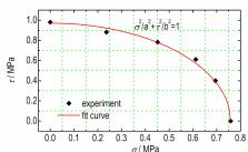
Mechanical properties of explosive crystal/binder interface in PBX were investigated by a new developed tension-shear method.
