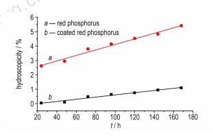
To reduce the hygroscopicity of red phosphorus, the red phosphorus was coated by aluminium hydroxide/phenol formaldehyde resin. The process of preparing the coated red phosphorus was optimized by orthogonal test. The coating layer of red phosphorus was characterized by FTIR and SEM.
