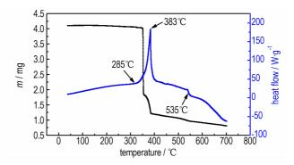
Potassium 5,5'-bistetrazole -1,1'-diolate(PBTOX) was synthesized by using glyoxime as starting materials. The structure of PBTOX was characterized. Its thermal behavior was studied by DTA-TG. The surface morphology and mechanical properties of PBTOX crystal were determined by atomic force microscopy(AFM) and Lorentzian contact resonance(LCR) imaging technique.
