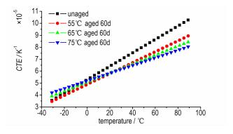
TU Xiao-zhen, SHEN Ming, ZHENG Chun, LI Lei Chinese Journal of Energetic Materials, 2016, 24(6): 614-617 The thermal expansion property of TATB based polymer bonded explosive(PBX) was studyed by high temperature accelerated aging test,  $\gamma$ and neutron irradiation test.
