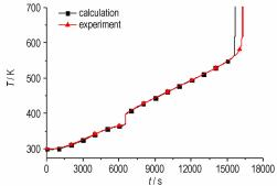
The cook-off bomb test of DNAN was carried out to measure the temperature variation and observe the reaction process inside the explosive. A thermal reaction model of fused cast explosive was established, and the phase transition process was described by using an enthalpy-porosity method.
