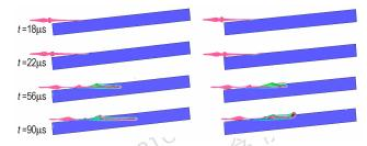
ZHAO Fang-xuan, SHEN Zhao-xin, LIU Ning, LI Ru-jiang Chinese Journal of Energetic Materials, 2016, 24(1): 33–37 The ricochet process of shaped charge jet penetration different material target, including 603 armor steel and aluminum, with a small incidence angle ranging from 5° to 7° was numerically simulated by using ANSYS/LS-DYNA software. Their penetration and ricochet process were observed.
