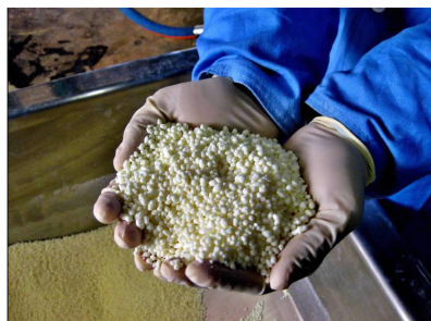
图2 HSAAP 制备含微晶蜡 (Indramic wax) IMX-104 造型粉颗粒
