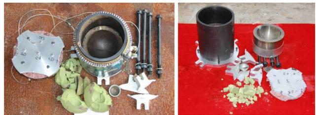
Fig. 6 Photographs of scrap in slow cook-off test of explosive components
