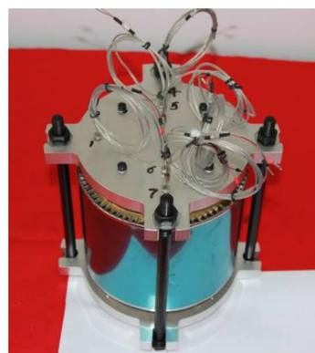
**Fig. 2** Photograph of slow cook-off test set-up with encased thermocouples and explosive components
