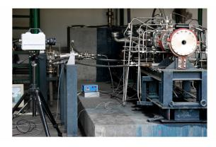
Boron based ducted rocket experimental system for ground simulation was established to study the boron combustion. Through heating the boron in a primary chamber by the combustion gas of the ethanol and oxygen, and using air react with boron in the secondary chamber, the working process under the condition of the flow field was simulated, and the similar condition for the real ducted rocket was obtained.
