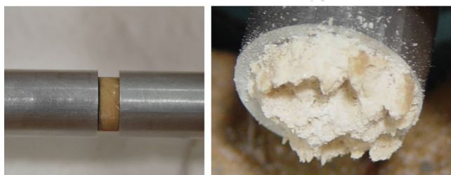
图 1 冲击前后 B-2 样品在 Hopkinson 杆上的状态 Fig.1 States of sample B-2 on the Hopkinson bar before and after impact
