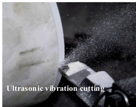
b. ultrasonic vibration cutting (UVC)
