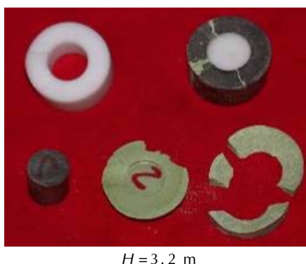
图 7 药片剪切试验中回收的 PBX-2 样品照片 Fig.7 Photographs of recovered sample for PBX-2 explosive in shear test
