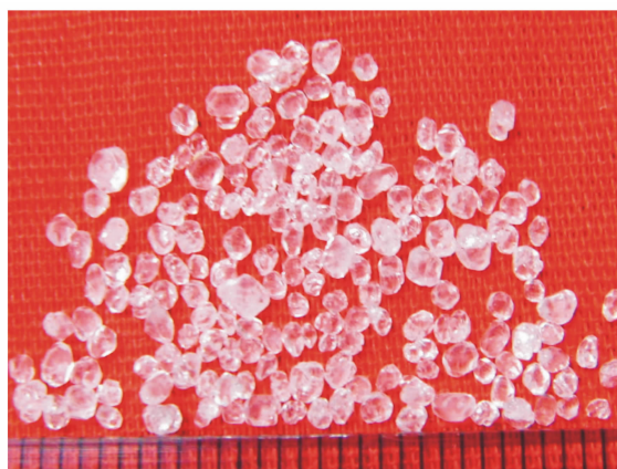
b. non-transparent normal quality particle RDX
