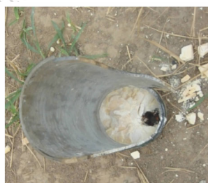
b. after -40 °C penetration test
