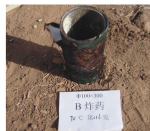
d. after 70 °C penetration test
