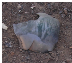
c. after 25 °C penetration test
